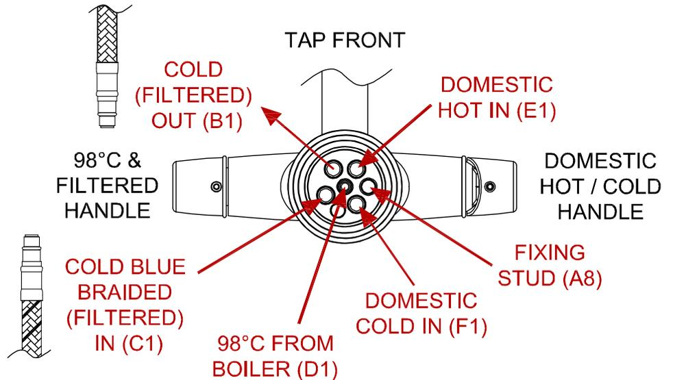
1. Screw the fixing stud (A8) into base of tap (A1) as shown on the diagram.
