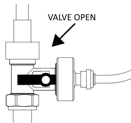
20. You can adjust the flow rate of the filtered water going to both the tap and boiler by adjusting the position of the blue lever on the isolating Tee valve (G7), you should aim for approximately 1-2 litres for both cold filtered and boiled filtered water.
