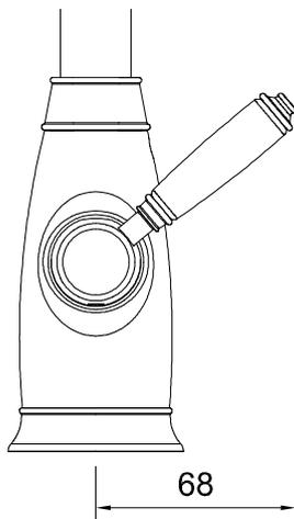
There needs to be a minimum 68mm gap between the tap hole centre and the back wall/splash.
