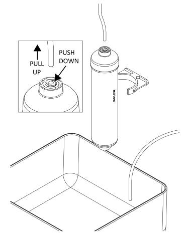
10. Push the "inlet" flexible blue pipe **firmly and fully** into the new filter cartridge inlet.
