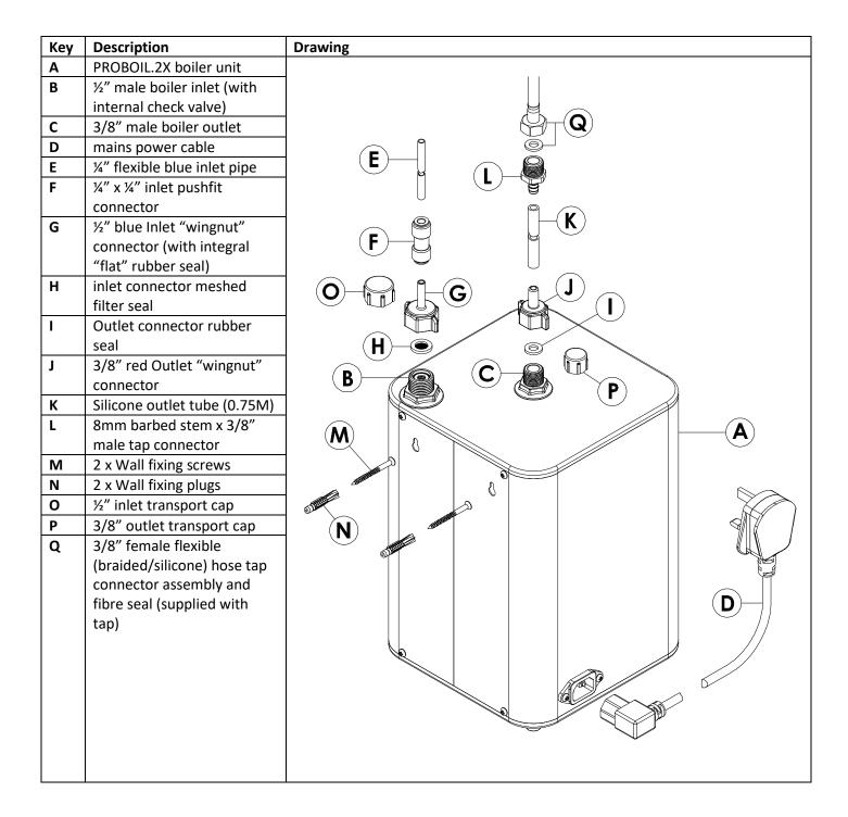
1. Roughly position the boiler (A) into its final installation location.
