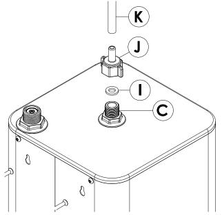
9) Remove the inlet meshed filter seal (H) from the boiler inlet (B) or inlet adaptor (G), rinse the washer in cold water, and use a toothbrush to clean any debris from it. If meshed seal (H) is compressed inside inlet (B) or adaptor (G) then use a cocktail stick (or similar) to remove it.
